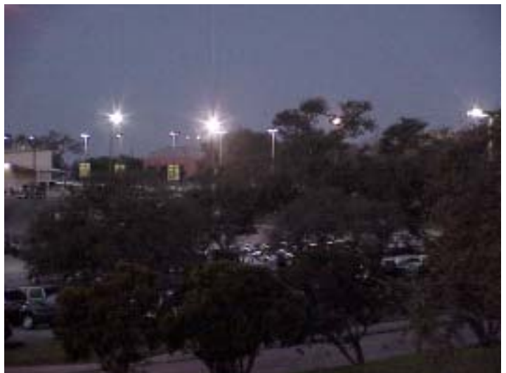
Example of commercial property with non-conforming lighting that produces glare and 'spill over' light onto adjacent properties
