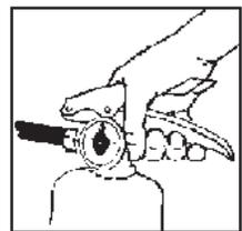
Squeeze the lever on the fire extinguisher.
